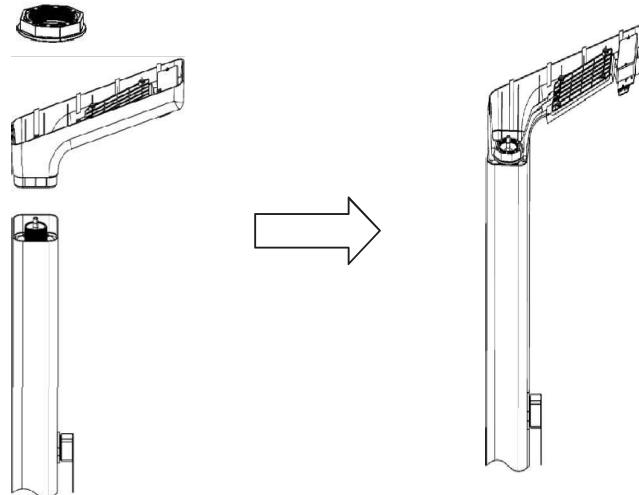
5. Install the water pipe, put on the circlip and tighten it with a screwdriver.
