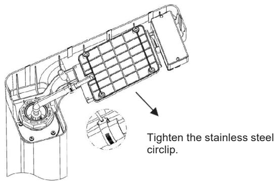
6. First insert the two connectors of the solar panel and the battery connector to the socket and then install the shower head cover.
