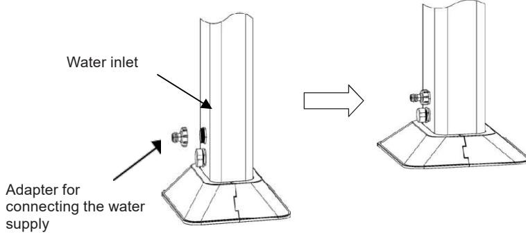
11. Prepare a hose with a closed water supply and connect it to the adapter for connecting the water supply.
